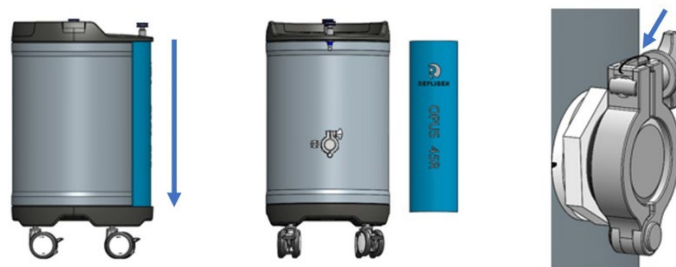
Figure 2. Sideguard and tie-wrap removal
